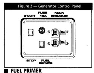
Before starting a cold engine (if it has not been started in more than two weeks), you must press this switch for approximately 5 seconds to bring fuel from the tank to the carburetor. This rocker type switch springs back into its original position when you release it.
